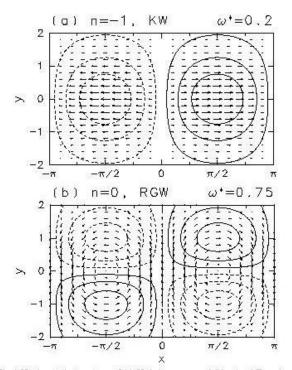
Fig.1 Horizontal structure of (a) Kelvin wave and (b) mixed-Rossby gravity wave. Contours show geopotential height component and arrows show horizontal wind components.
